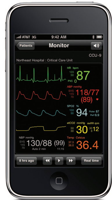
Fig. 1. Airstrip Technologies remote continuous vital sign monitoring via the iPhone. This software delivers real-time data about the vital signs (including blood pressure, heart rhythm and rate, blood oxygen level, and body temperature) of any patient who is in a hospital intensive care unit to a doctor's or nurse's smart phone.
